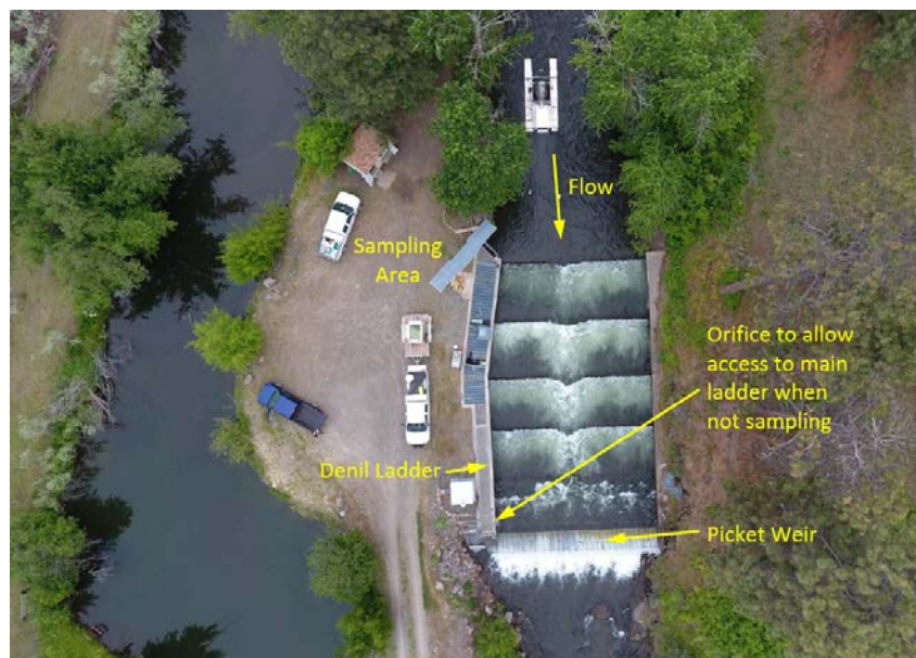
Figure 2: Aerial view of Weir and Fish Ladder
